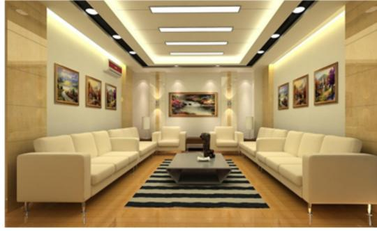
False ceiling is provided below the roof slab on suspended supports. The false ceiling is usually provided for temperature control (heat insulation for AC), to install lights, or to conceal electrical and other networking cables and ugly or too high ceiling.
